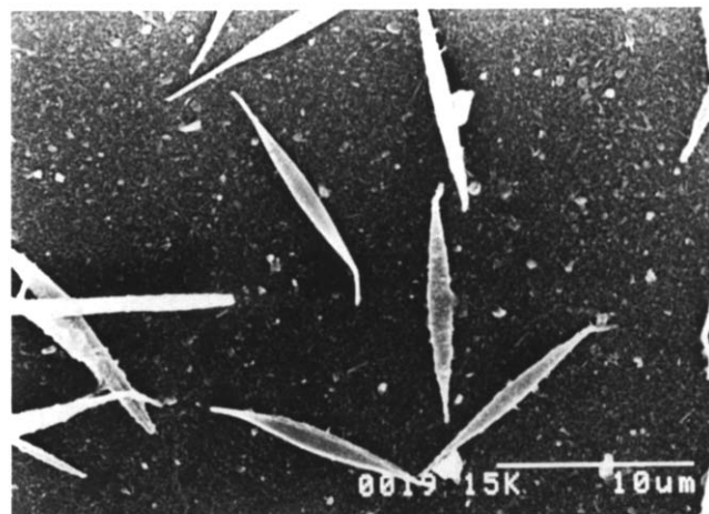
Figure 3 Scanning electron micrograph of PON crystals prepared in TS 800 (PON-2)
